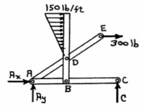
From a free-body diagram for bar ABC: +  $\zeta \Sigma M_{A} = B_{y}(4) + 495(10) = 0$  $B_{y} = -1237.5 \ 1b = 1237.5 \ 1b \downarrow$
