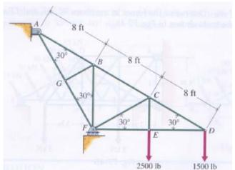
b) (15 Points) Determine the forces in members BC, CF and EF of the truss shown. Hint: use METHOD OF SECTIONS SOLUTION
